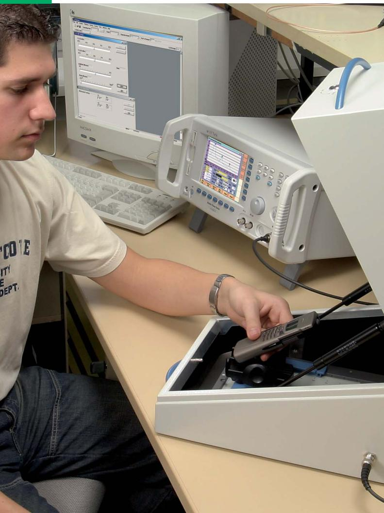
Connect the 4400 to a remote PC to upload and post-process measurement results
